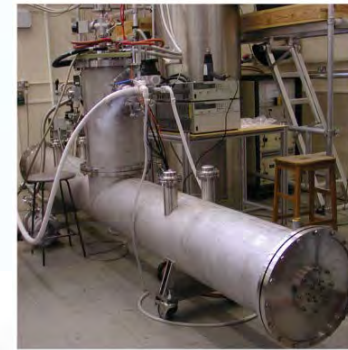
Two undulators in one cryomodule were tested at Daresbury. Both achieved nominal magnetic fields.
