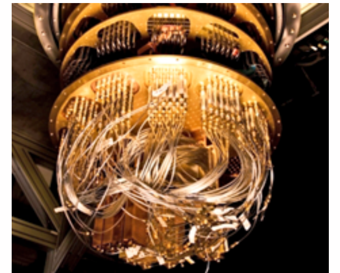
Google's dilution fridge cabling
