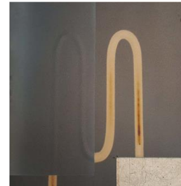
Integrated radiation-hard heating track
