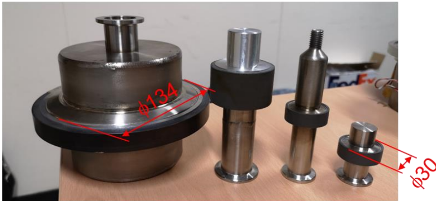
SMA connectors (up to DN100) suitable also for bimetallic junction
