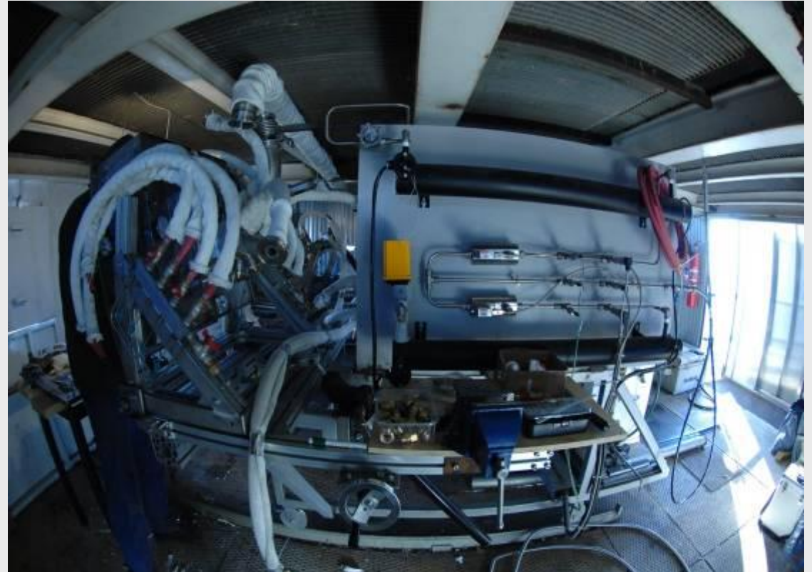
The HYDROSOL II reactor on the SSPS tower
