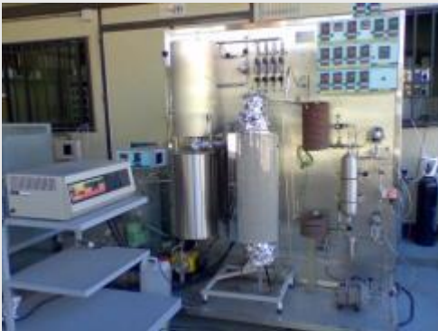
Pilot membrane gas separation plant
