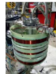
Helmholtz coil for cavity vertical test
