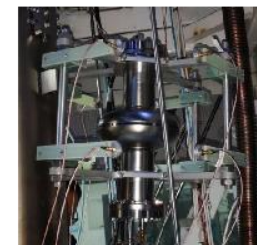
Second sound cavity quench detection system
