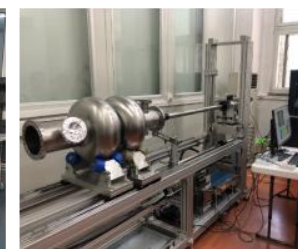
Cavity inspection camera and grinder
