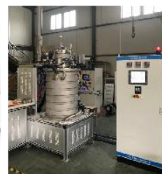
Nb 3 Sn furnace
