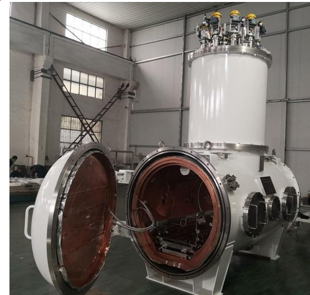
General superconducting cavity test cryomodule in IHEP New SC Lab
