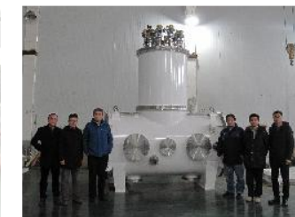
Horizontal test cryostat
