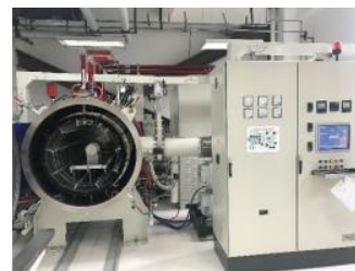
Vacuum furnace (doping & annealing)
