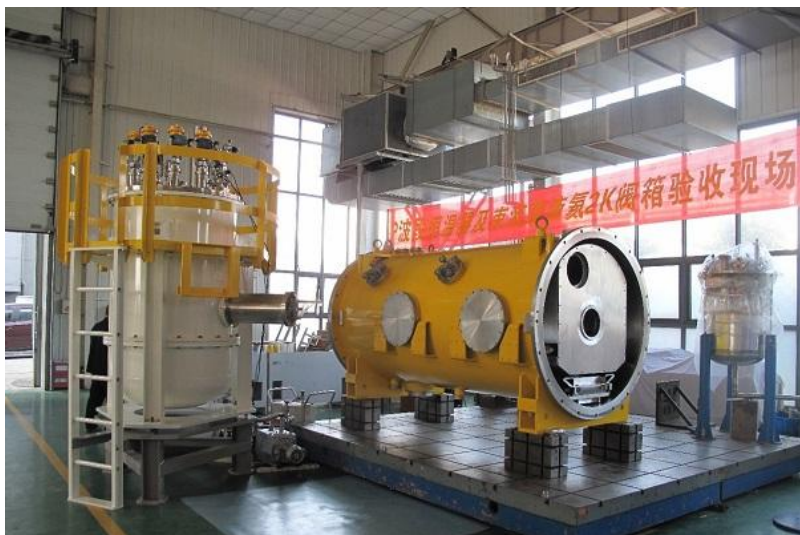
CEPC 2*2cell 650MHz cryomodule with beam test later
