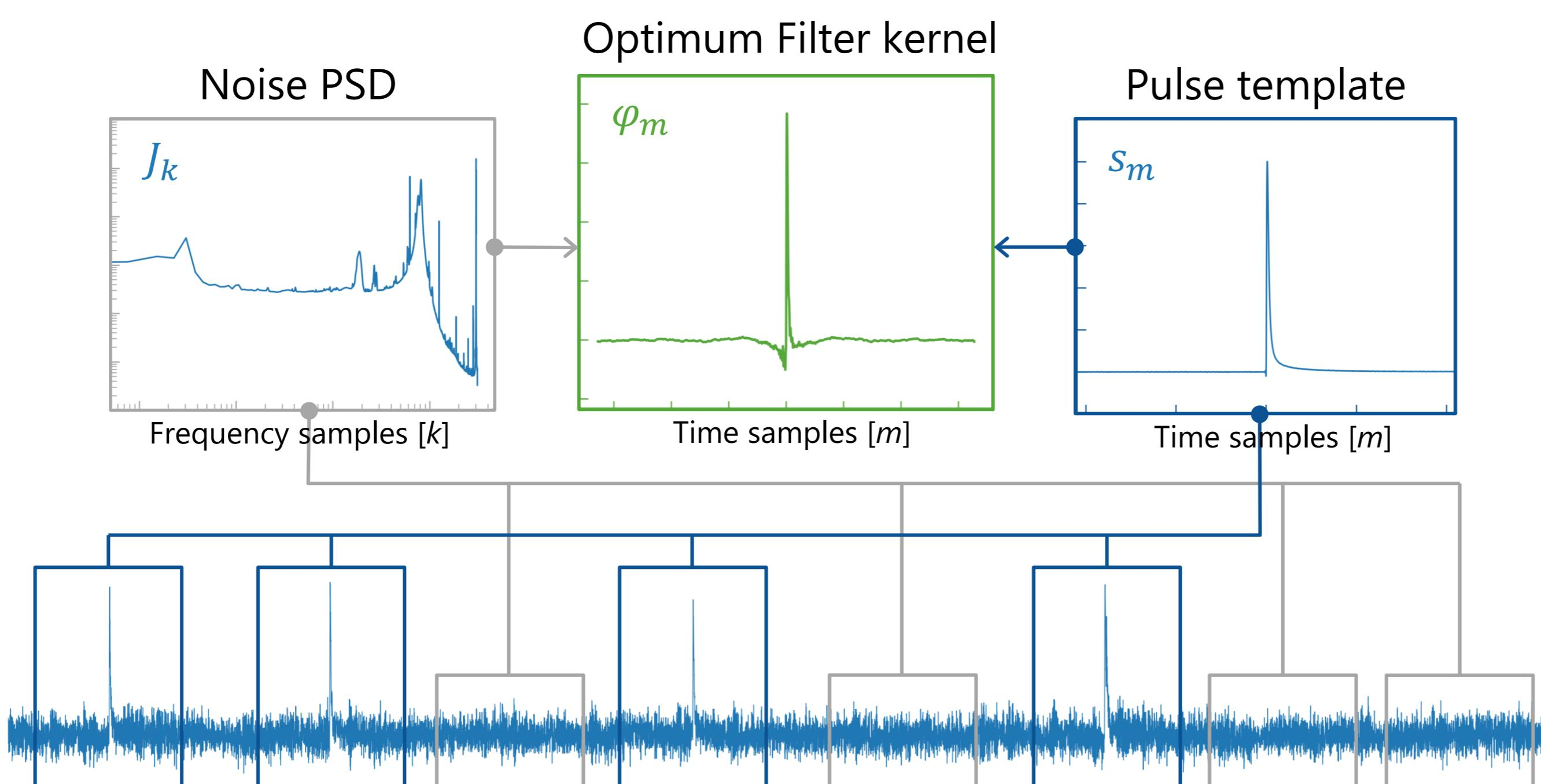
$J_k$  – noise Power Spectral Density (PSD)
