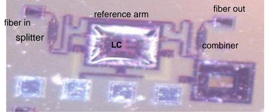
As can be seen in the picture on the left, liquid crystal is applied locally to the chip. This is possible because of an etched cavity (hole) in the chip surface.
