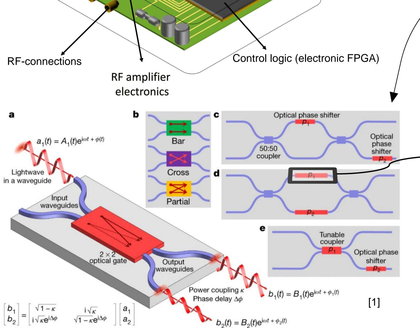
The waveguide mesh connects 2x2 optical (analog) gates together in hexagons. a) These 2x2 gates can take light from any input waveguide and couple it to any of the two output waveguides b) There are 3 states possible in one of these gates. In c), d) and e) different possible implementations of such gate are shown.
