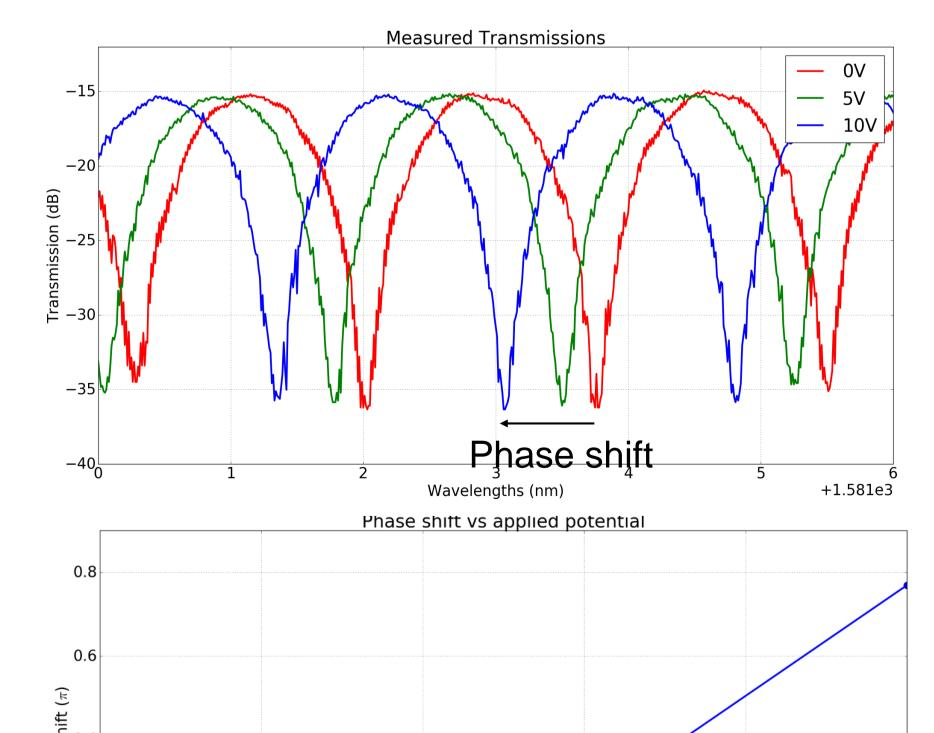
The spectrum of the interferometric circuit is measured for each voltage. The phase shift can be found in the shift of the spectrum of this measurement.
