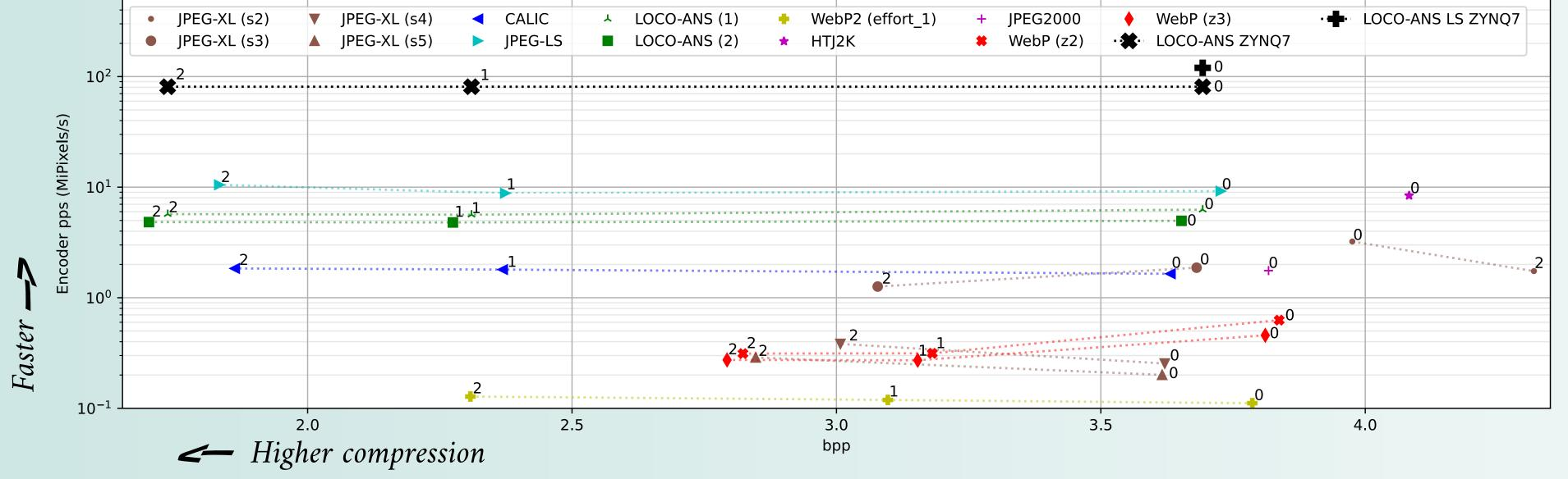
Peak error shown next to performance point. Software implementations were run in a Raspberry Pi 3 Model B. Preliminary hardware codec was implemented in a ZYNQ 7010/20.
