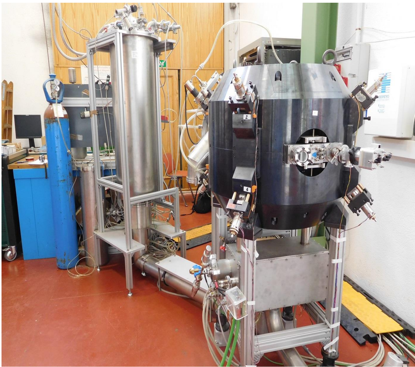
Fig. 1. AMIT superconducting cyclotron and the cryogenic supply system (CSS).
