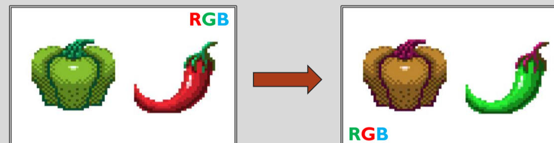
Figure A: visual representation of the 1SA protocol: one image is selected (1), from which two randomly selected channels are swapped (S), for all pixels (A) in the image.
