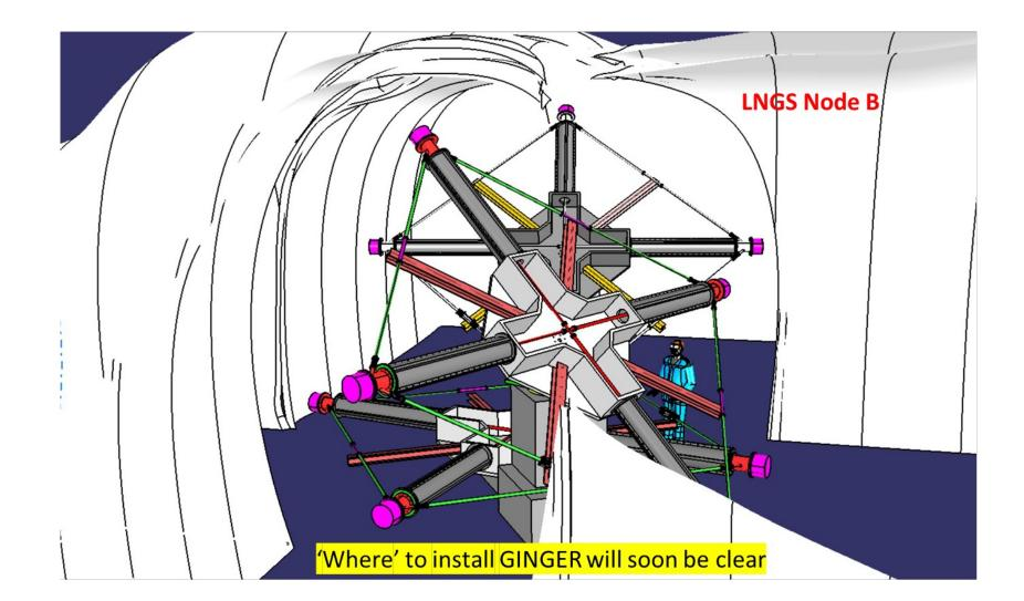
Array of 3 ring laser gyroscopes (RLG), 5m sides, the drawing is related to Node B of LNGS This area is large enough to separate most of the electronics in a separate room.
