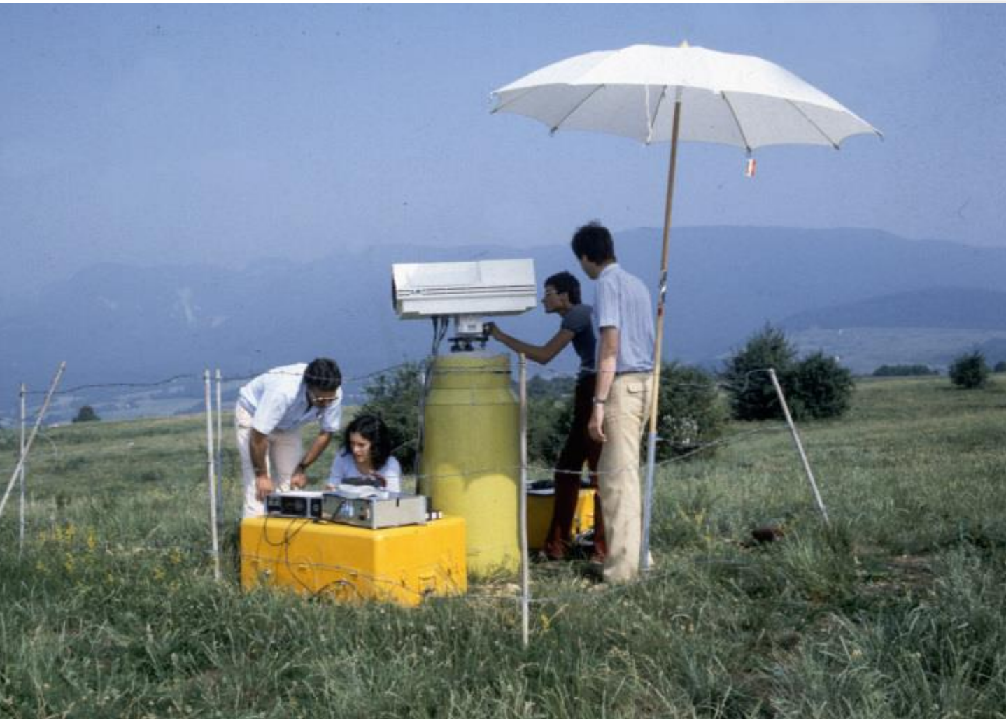
Distance measurements between geodetic pillars using terrameter
