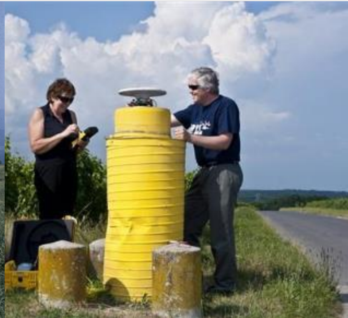
GNSS measurements on a Geodetic pillar
