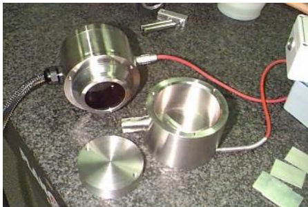
Hydrostatic Levelling Sensor (capacitive-based)
