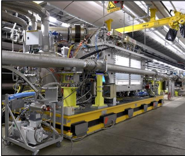
Crab cavity prototype installed in SPS
