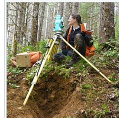
A surveyor using a total station
