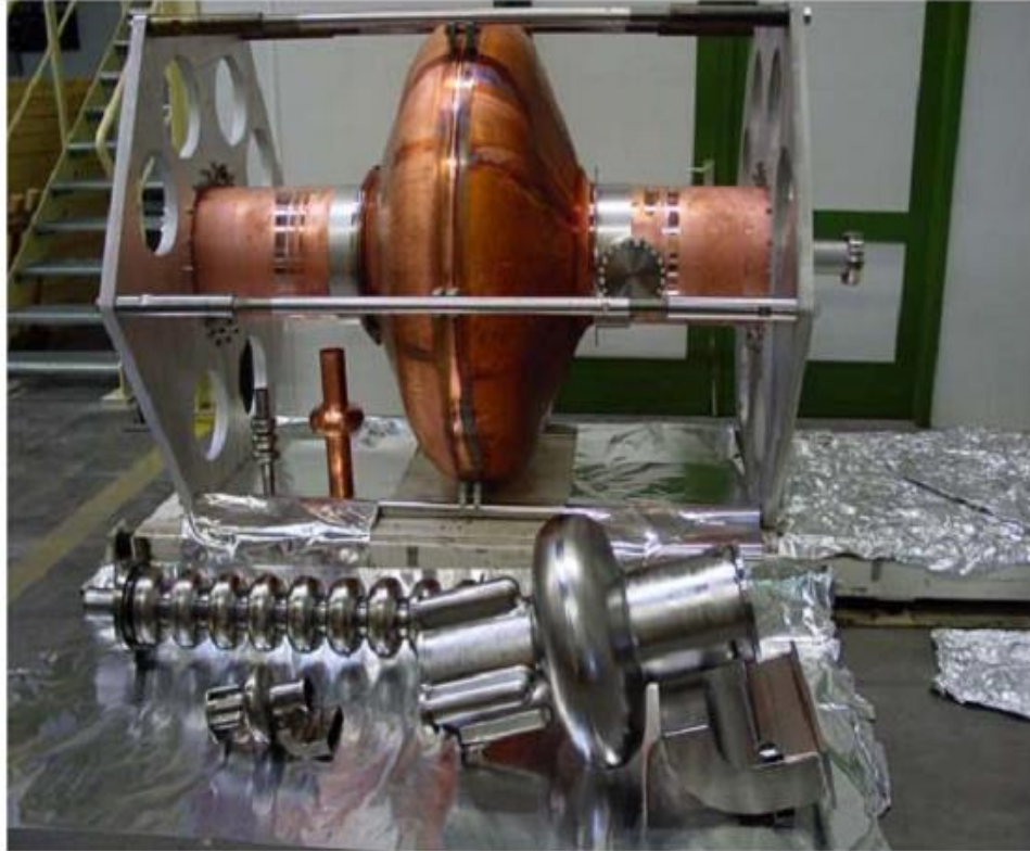
Fig. 1 A spectrum of superconducting cavities.
