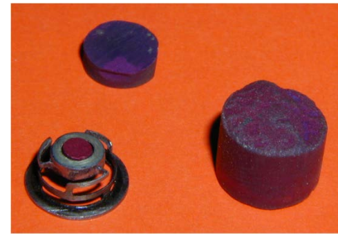
cathodes damaged by sputtering
