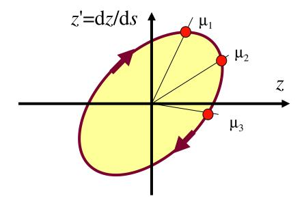
In the case of a ring or matched cell, the periodicity imposes equality on the input and output  $\alpha$  and  $\beta$  values. This means that the particle returns after each turn or transit to the same ellipse but at phases  $\mu_1=B$ ,  $\mu_2=B+2\pi Q$ ,  $\mu_3=B+4\pi Q$ , ....,  $B+n2\pi Q$  and so on.
