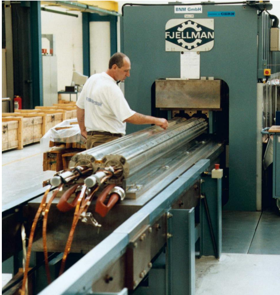
Collaring of a dipole magnet
