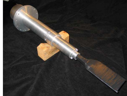
Figure 2.30: Left: The scheme of a plastic scintillation counter connected to the photo-multiplier via a plastic light guide. Right. Photo of scintillator wrapped in black tape and the base in within the metal housing.
