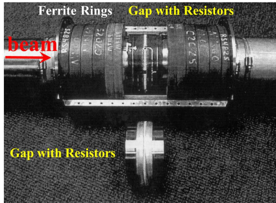
Figure 6.14: Photo of the wall current monitor used at FERMI-Lab for protons, from [131]. The ceramic gap is shown separately. The ferrite rings and the printed circuit with the resistors are visible.
