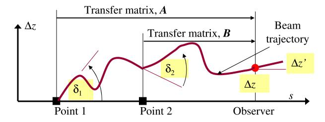
**❖** The system is linear, so the effect of each kick at the Observer can be calculated and the effects added.
