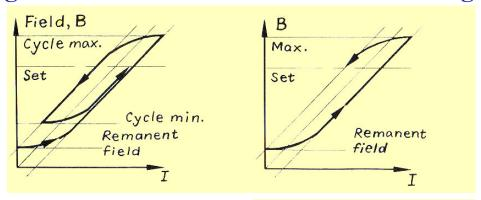
When accelerating the beam, slow dI/dt to prevent overshoot (rst control loop).
