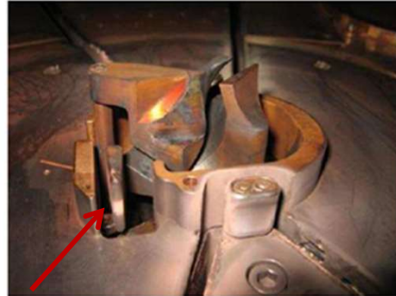
An additional horizontal deflector is needed for multi-particle cyclotron
