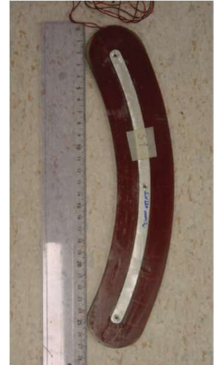
Example of a harmonic coil
