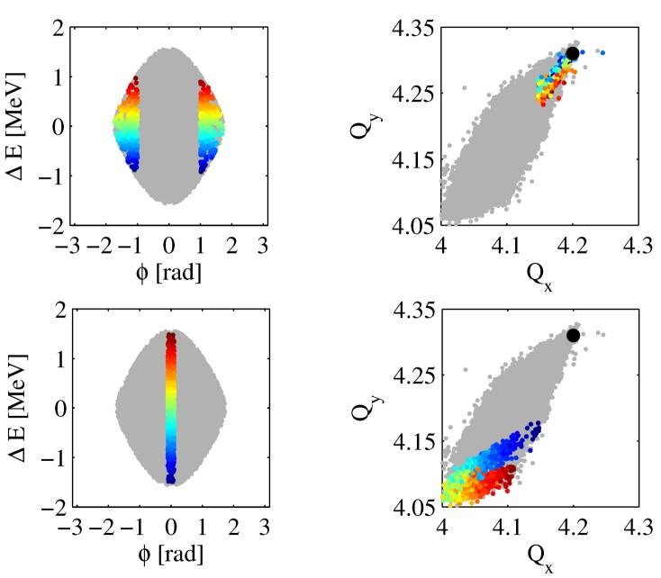
Longitudinal phase-space  $(\Delta \phi, \Delta E)$  scatter plot of the bunch tune footprint. The black dot is the bare tune. Particles at the edges of the bunch have tunes close to the bare tune in the necktie.
