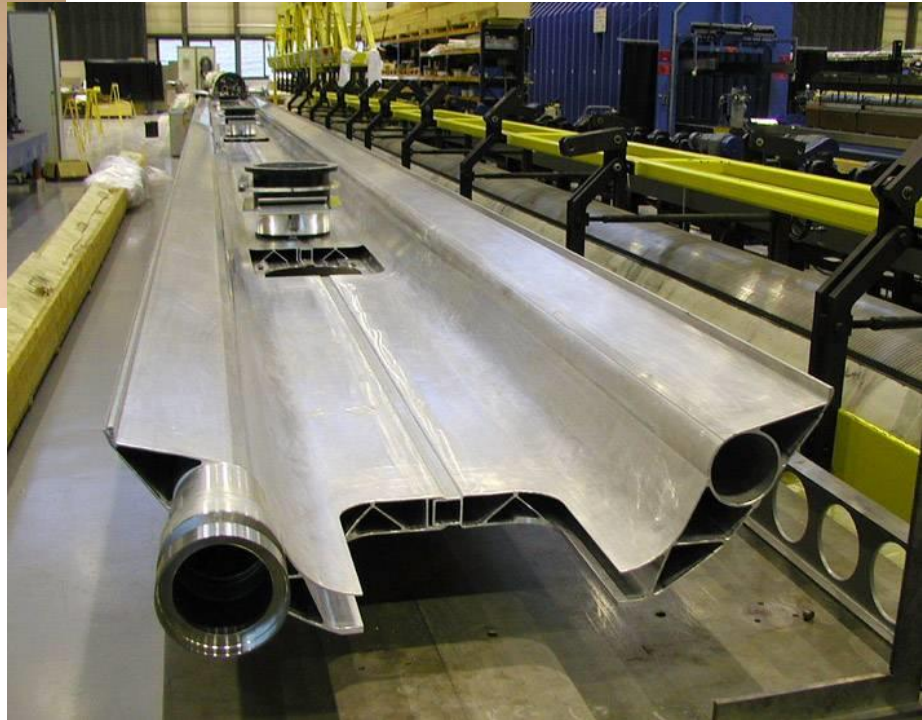
Aluminium extrusion for thermal shield
