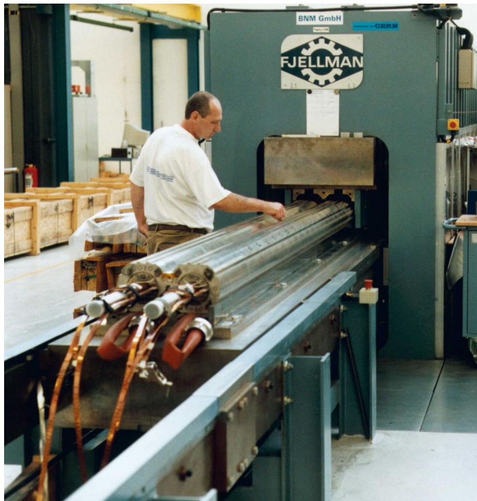
Collaring of a dipole magnet
