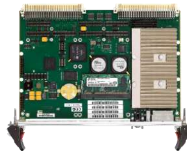
VME Card: Eurocard size VMEbus interface
