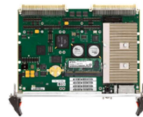
VME Card: Eurocard size VMEbus interface
