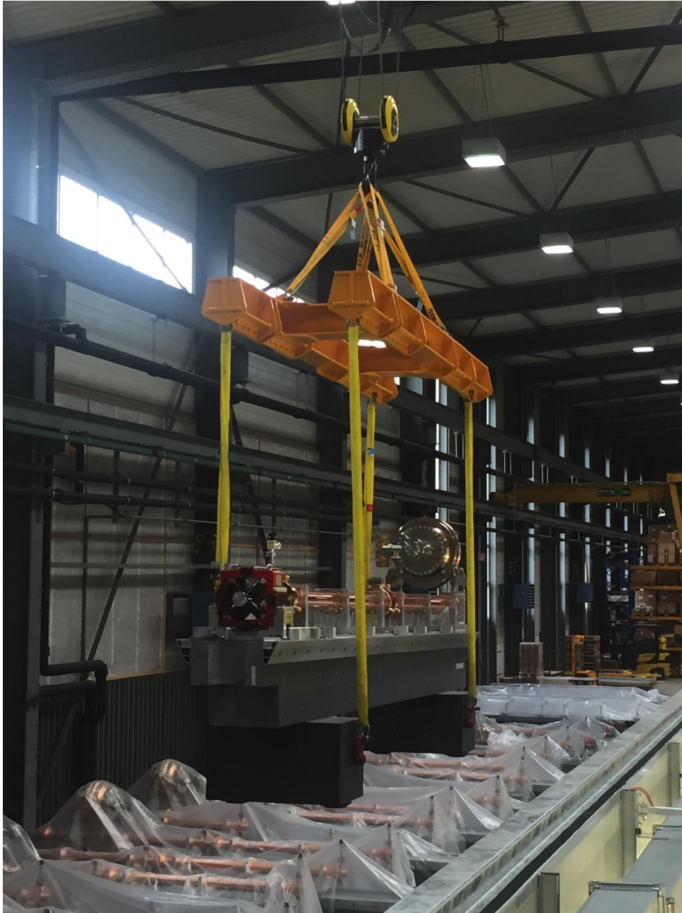
Movement of girder into assembly hutch
