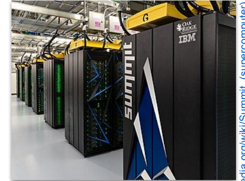
Summit Supercomputer: 4608 nodes. Per node, 2 IBM POWER9™ CPUs, 6 NVIDIA V100 GPUs.
