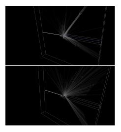
• Screen changes angle as a function of position along length, so that different part of the Cherenkov light cone escape, constraining detection by input angle as well as position
