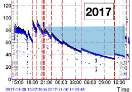
As the luminosity drops, turn on various single-muon  $|\eta|$ -restricted seeds, which allow to keep L1 rate constant and increase HLT rate toward the end of
