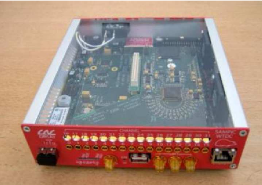
16 channel SAMPIC (D. Breton, J. Maalmi et al.)
