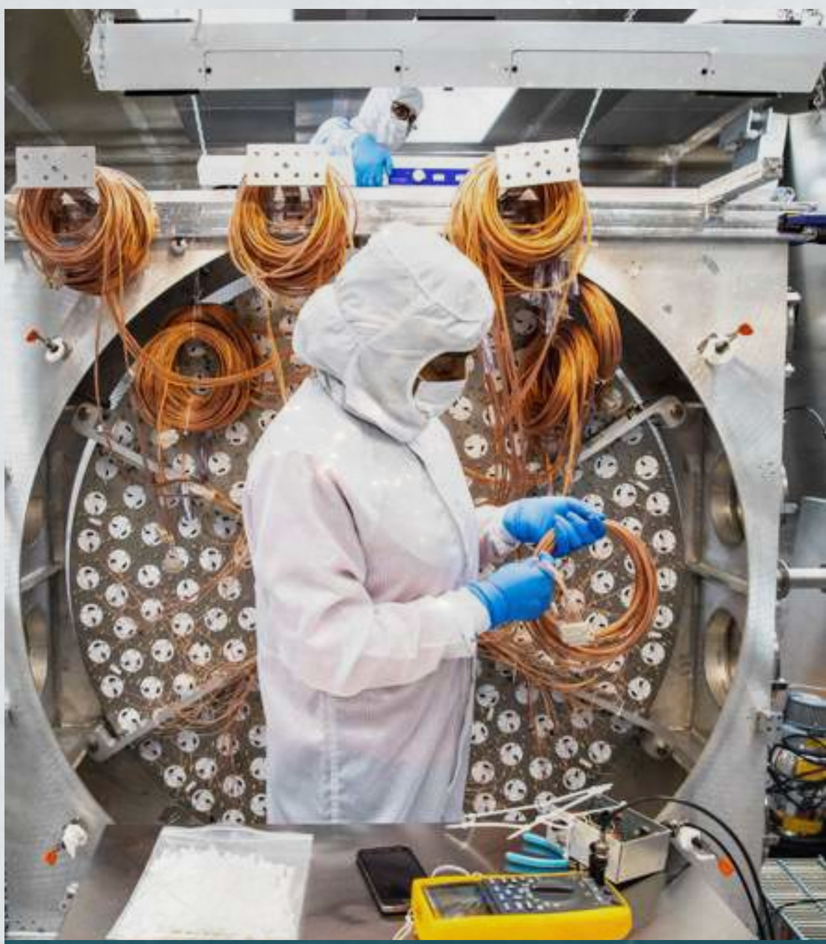
PMT array cabling at SURF
