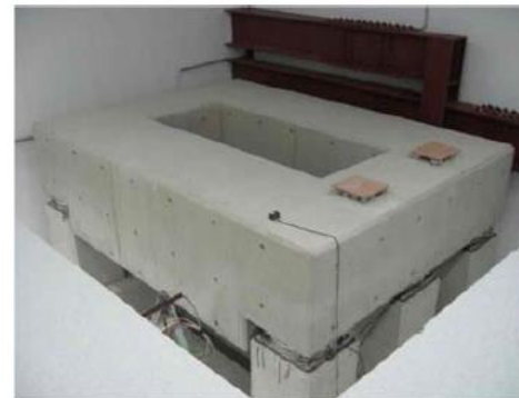
Figure I-7: Vibration transfer characteristic curves and Low vibration block(LVB) & air-type passive vibration isolators of manual anti - vibration dampers
