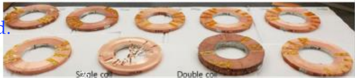
Figure 2.67: Manufacturing process (10 HTS coils)
