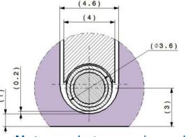
**Note gap** between wire and tungsten (0.1÷0.2 mm)
