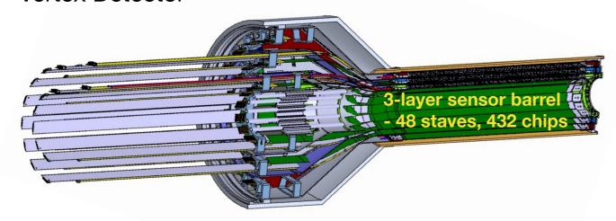
Service cone: signal, power, cooling and mechanical support
