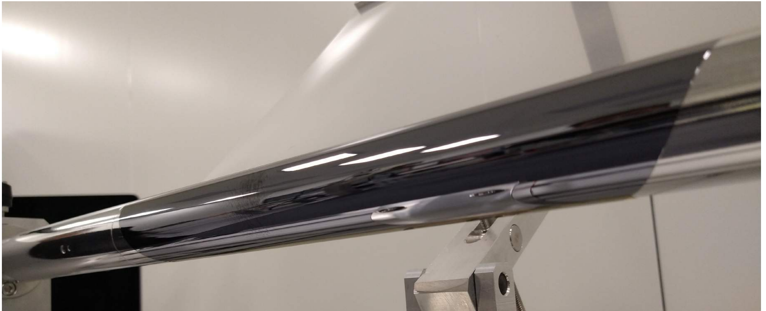
Bent silicon piece kept in position with Kapton adhesive tape
