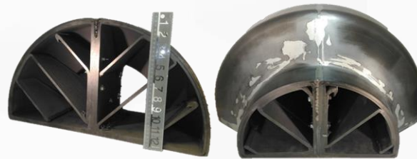
Finished tool surface coated with mold release
