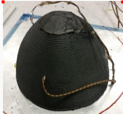
Printed blackbody cavity equipped with temperature sensors
