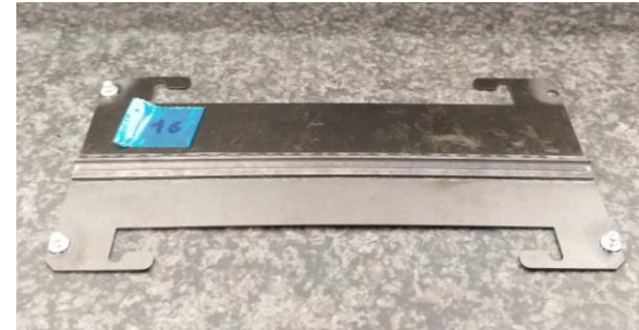
Sintered Al-CF (MB): Deformation from 0.35mm to 0.80mm
