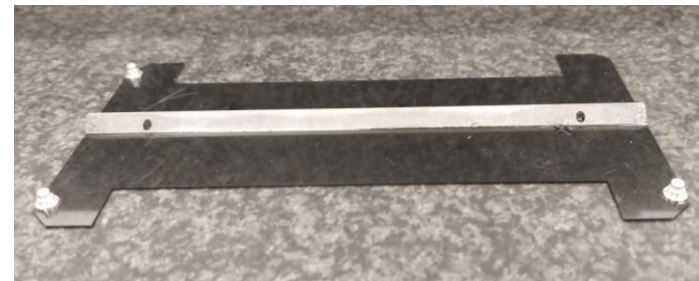
Casted Al-CF (MA): No visible deformation
