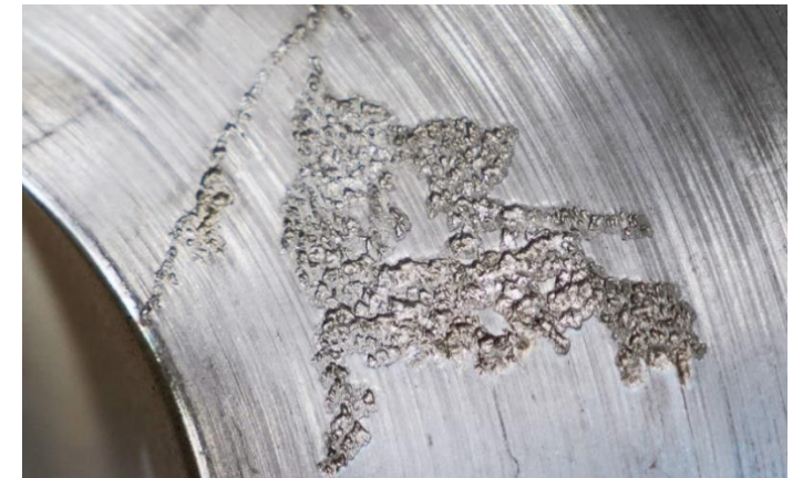
Hydro-mechanic machinery damaged by hydrodynamic cavitation
