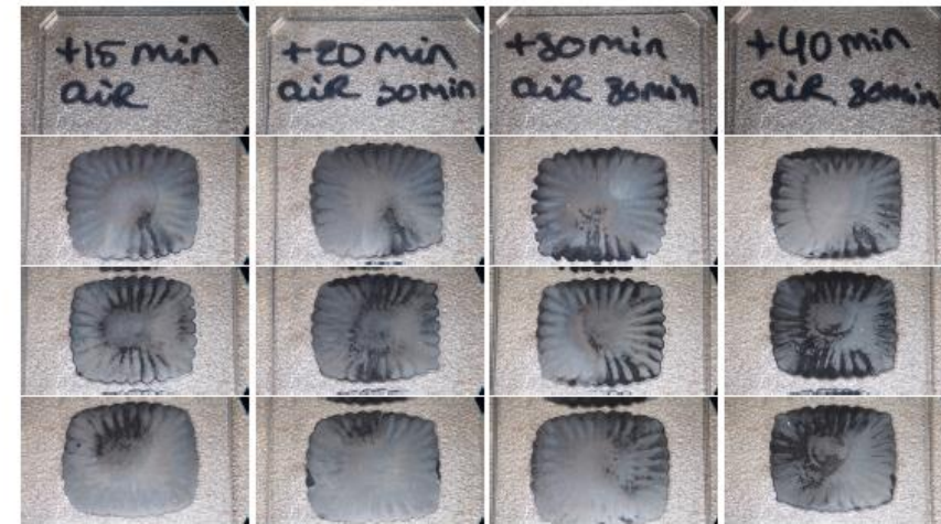
Figure 32: Samples produced at different working points and pressed after 30 minutes in the clean room. Photographed after curing and ageing for 284 hours at 70°
