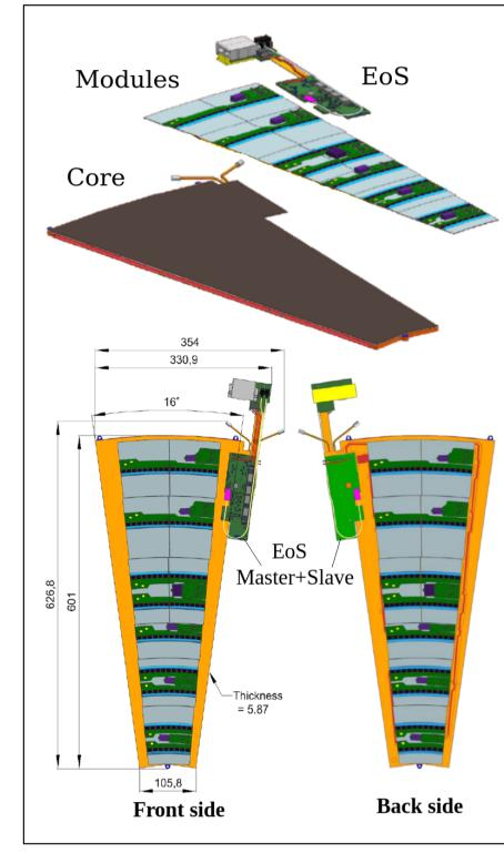
» the **petal** consists of the local support structure, the core, the directly glued on sensing elements, the silicon strip **modules**, and the also glued on offdetector interface board, the **end-of-substructure** » the petal concept follows a **modular approach** for the assembly of components and minimizes the **material budget** of the detector (e.g. direct gluing, wire-bonding) » the wedge-shaped **petal core** is a light-weight sandwich structure and provides:
