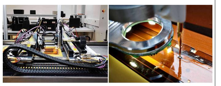
**Thermal performance check** » IR thermography on petal core
