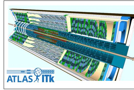
» the ATLAS Inner Tracker (ITk) will replace the current tracking detector in the **HL-LHC** phase to cope with the challenging conditions (radiation, pile-up) » the tracker is an **all-silicon** detector with **pixel** and **strip** detectors arranged in a central **barrel** region and two **endcaps** in the forward regions
