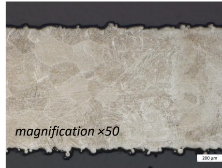
after etching – grain size can be appreciated
