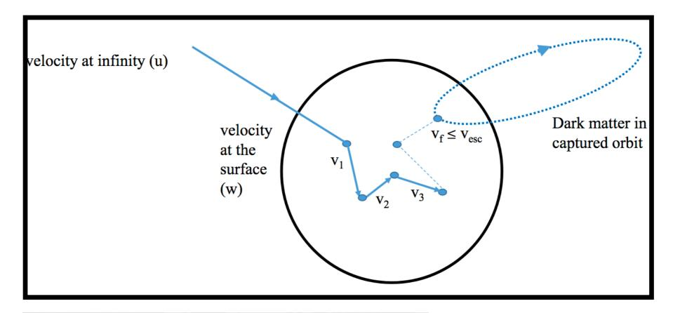
$$C_N = \underbrace{\pi R^2}_{\text{area of the object probability for }N} \times \underbrace{p_N(\tau)}_{\text{area of the object probability for }N} \times \underbrace{n_{\mathrm{DM}} \int \frac{f(u)du}{u} (u^2 + v_{\mathrm{esc}}^2)}_{\mathrm{DM flux}} \times \underbrace{g_N(u)}_{\text{probability that }v_f \leq v_{\mathrm{esc}}}_{\text{after }N} \text{ collisions}$$
