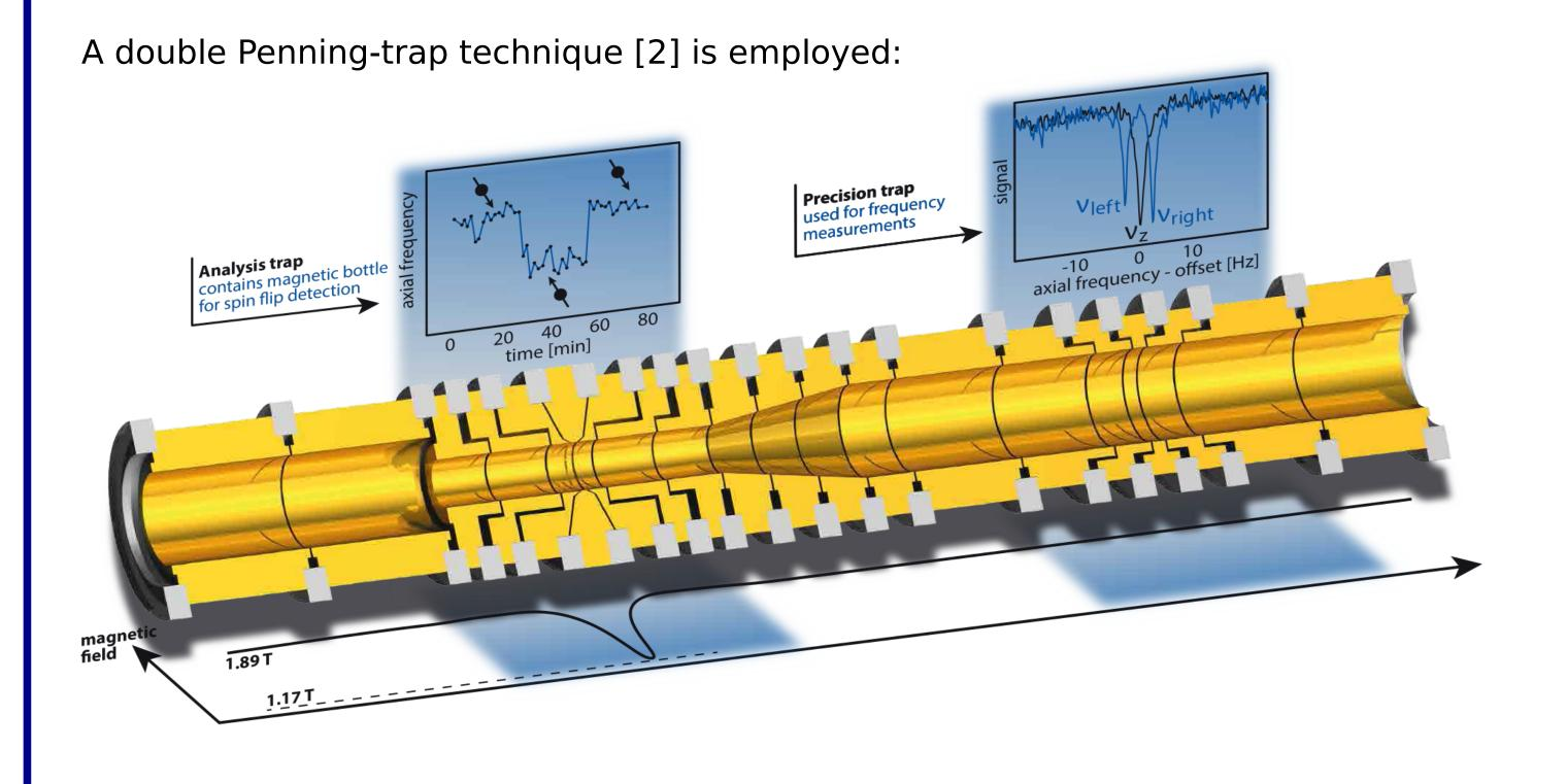
In the precision trap, all the frequency measurements are performed. While the axial frequency is determined directly, the modified cyclotron frequency is measured by applying an electrical field close to  $\omega_+ - \omega_z$  This couples the frequencies and results in a double dip spectrum from which  $\omega_+$  can be calculated. The determination of  $\omega_-$  works analogously.
