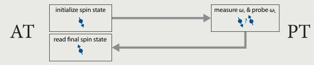
Application of a drive at the excitation frequency  $v_{rf}$  and simultaneous measurement of the cyclotron frequency  $v_c$  in the precision trap yields the ratio  $v_r/v_c$  and probes the *g*-factor resonance (the spin-flip probability as a function of the ratio  $v_{rf}/v_c$ ).
