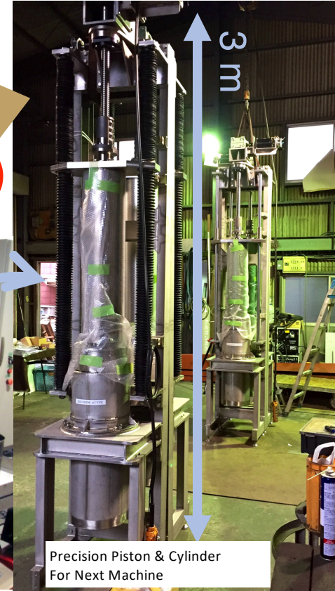
3rd Machine (under construction) 10 m 2 /Operation →2000-3000m 2 /year
