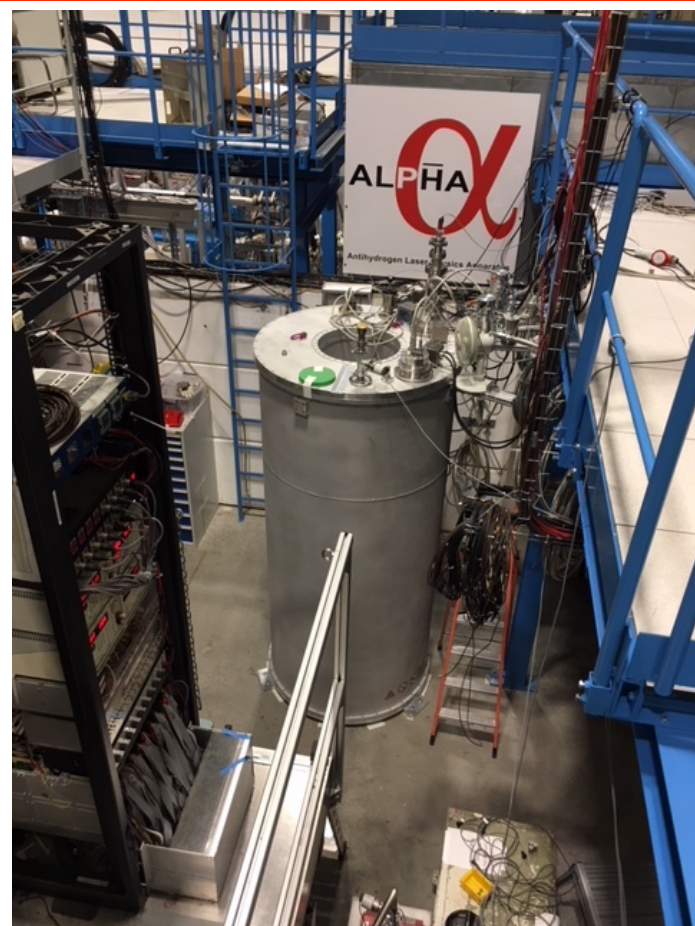
external solenoid to be shimmed
