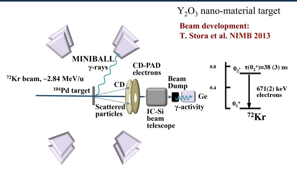
Electron detection from the decay of second  $0_2^+$  state in <sup>72</sup>Kr using a CD-PAD detector
