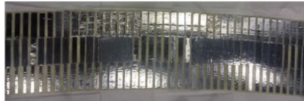
Fully-assembled lamination (10 degrees wide)
