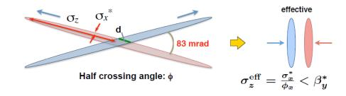
Strong focusing of beams down to vertical size of  $\sim$  50 nm requires very low emittance beams and large crossing angle (83 mrad)  $\Rightarrow$  Need powerful and sophisticated final focus system (QCS) beam currents are also increased by a factor 1.5
