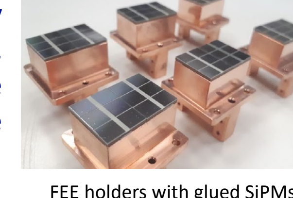
FEE holders with glued SiPMs
