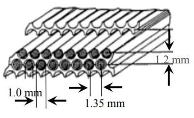
Sampling EM calorimeter: lead + 1mm scintillating fibers
