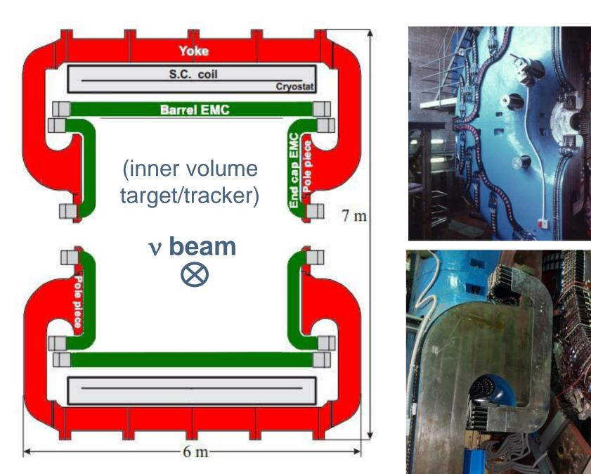
The **ECAL** is divided in a cylindrical barrel section, made of 24 trapezoidal 4.3 m long modules, and two endcaps, each with 32 differently-sized "C"-shaped modules, to achieve a  $4\pi$  total acceptance. The fibers are grouped in cells and read on both sides. The ECAL combines a fine-structure and excellent energy and time resolution.
